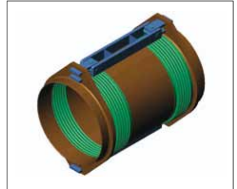
3D Drawing of a multiplane, hinged expansion joint - for angular movements.
