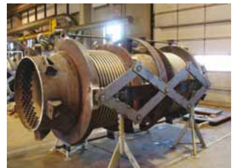
Metal expansion joint with refractory lining, in process.
