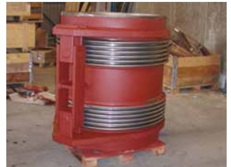
Multiplane, hinged expansion joint - for angular movements.
