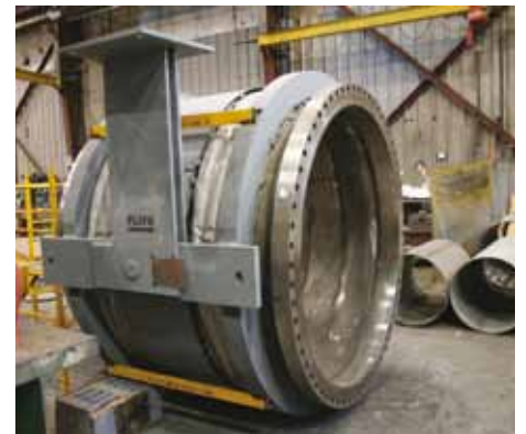
DN2000 (72" ) Hinged Expansion Joint for a Turbo Expander Piping System.
