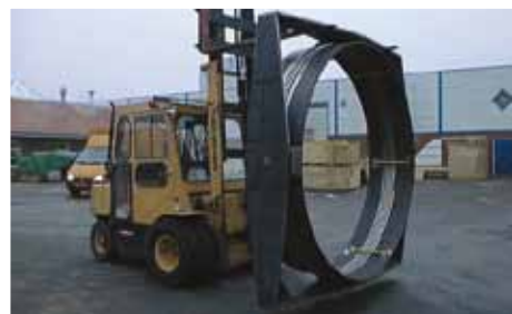
Multiplane, angular expansion joint with gimbal.
