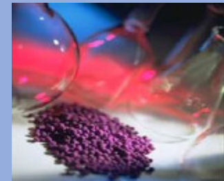
Dry scrubbing media
